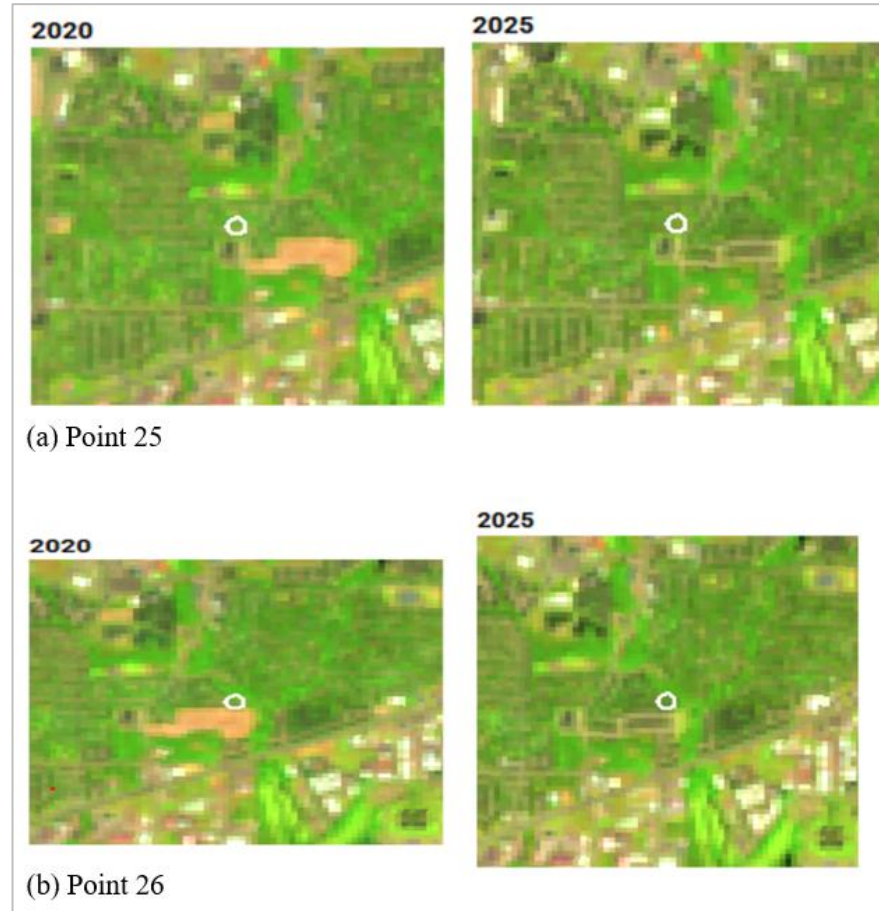
Figure 3. Landsat Time Series Explorer visualization showing temporal vegetation dynamics at points 25 and 26 within the AOI. The imagery compares vegetation and canopy conditions across multiple time intervals over a five-year period, highlighting localized stability and variability in vegetation health within residential zones.
