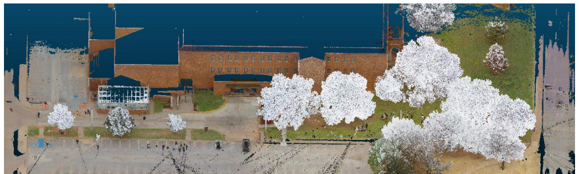
Figure 2. Sample LiDAR scan showing tree point clouds on the south side of Bolin Science Hall.
